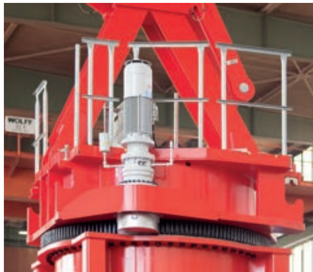
Detailed view: Slewing gear of a rotating tower crane
