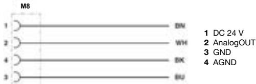
Example for standard cable: SAC-4P- 2,0-PUR/M 8FS 0,34 – sensor/actuator cable (Phoenix Contact)
