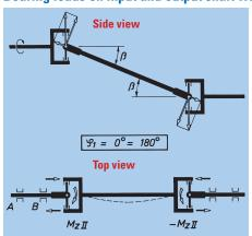
Driveline-center part stressed in bending
