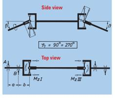
Input and output shaft stressed in bending
