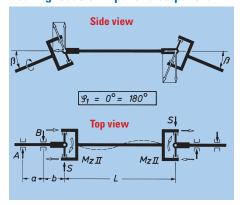
Input and output shaft stressed in bending
