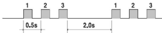
Figure 10-1: Alarm blink signal.
