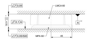
\* The stated mounting height is set for the air gap of 0,6 mm. For more information, please refer to the Linear Motors catalogue. \*\* We recommend using a thermally conductive paste between the forcer and heatsink to ensure a better heat transfer.
