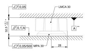
\* The stated mounting height is set for the air gap of 0,6 mm. For more information, please refer to the Linear Motors catalogue. \*\* We recommend using a thermally conductive paste between the forcer and heatsink to ensure a better heat transfer.
