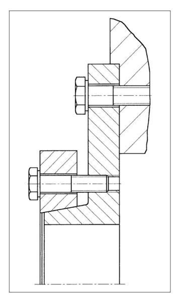
The flange is supplied with a tolerance of D-0.1 mm and can therefore be used to spigot pulley end plates or other driven components.
