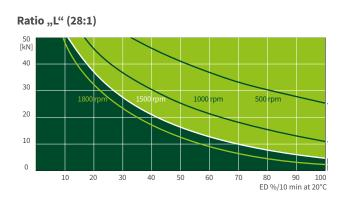
These curves are for guidance under standard industrial conditions (ambient temperature 20°C etc.) and correct maintenance (lubrication etc.). They are based on the ZIMM standard trapezoidal thread Tr 40x7. With the use of a ball screw, the operation cycles can be many times longer.
