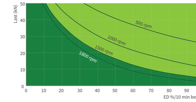
These maps are for orientation under standard industrial terms (ambient temperature 20% etc.) and proper maintenance (lubrication, etc.). They are based on the ZIMM standard trapezoidal thread Tr 40x7. With the use of a ball screw, the operation cycles can be many times longer. In case you need an even longer duration or performance, you will find information about our ZE-H high performance gearboxes on chapter 2.3.
