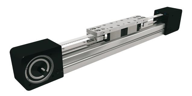
The aluminium profiles are manufactured according to the medium EN 12020-2 standard Straightness = 0,35 mm/m; Max. torsion = 0,35 mm/m; Angular torsion = 0,2 mm/40 mm; Parallelism = 0,2 mm
