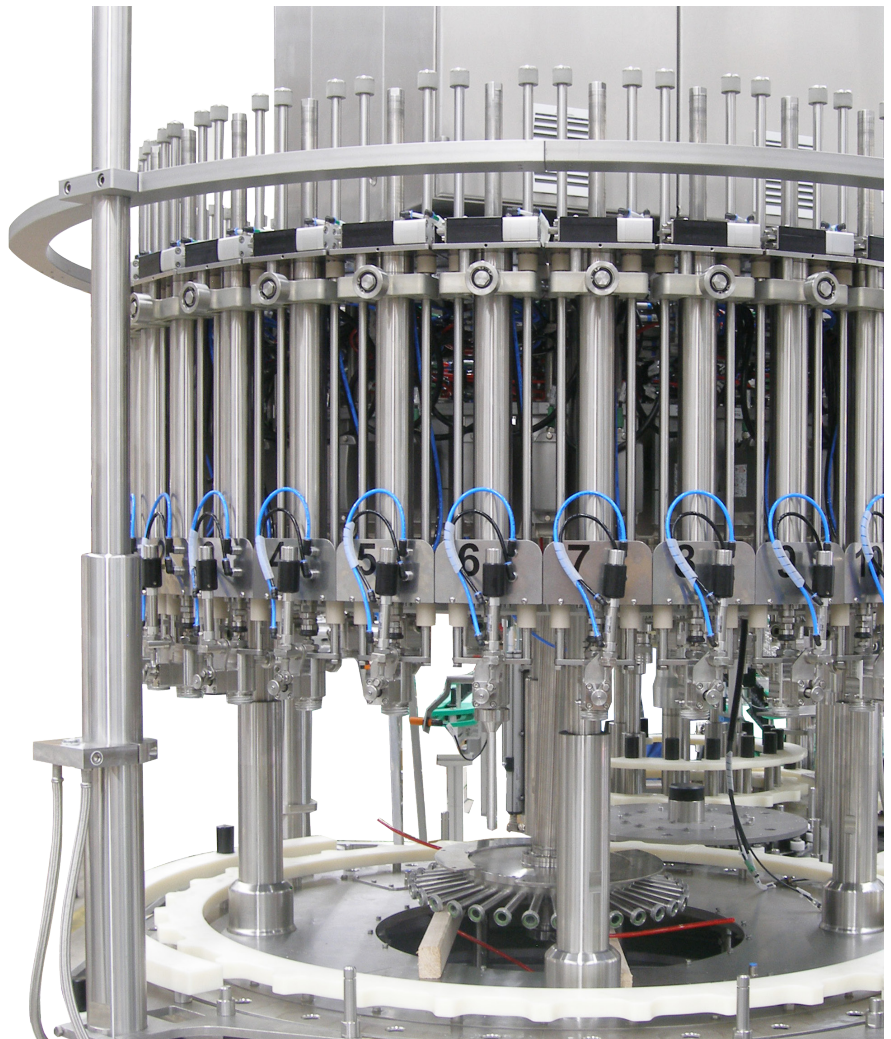
The monoblock system has space for 36 filling stations, in which each filling needle is driven by a LinMot linear motor. This allows rapid product changeover and broadens the range of application of the filling and closing machine. (Photo: Rossmann)
