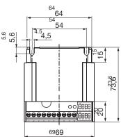
Accessories: Mounting bracket set for 35 mm rail acc. EN 60715: Article No. 1802911
