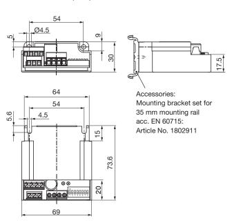
Through the monitoring of different parameters, the ROBA®-brake-checker recognises safety critical operating conditions of the brake in advance, as well as acute faults (e.g. line breakage). These are determined as they occur and are notified to the user as a warning before the brake can no longer be operated.
