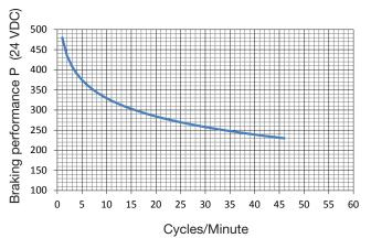
For brakes, which do not require overexcitation, the holding voltage may be lower than the nominal voltage, e.g. on power reduction to reduce the coil temperature.
