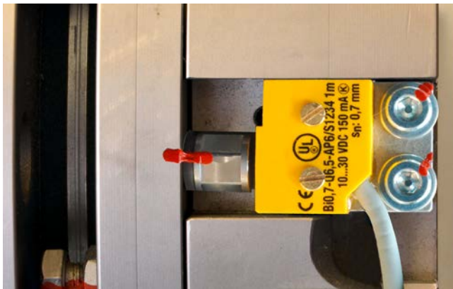
Contactless release monitoring with inductive proximity switches
