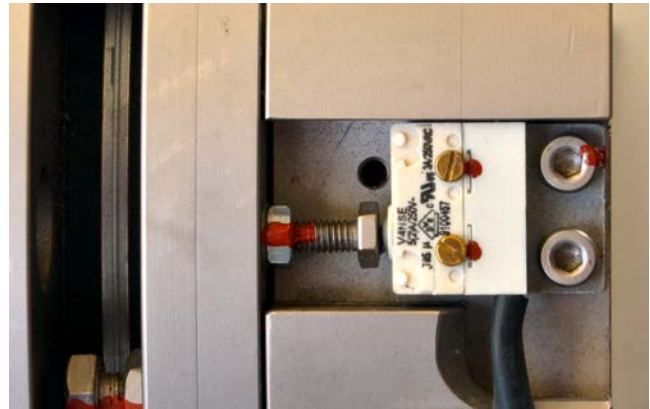
Release Monitoring with Microswitch
