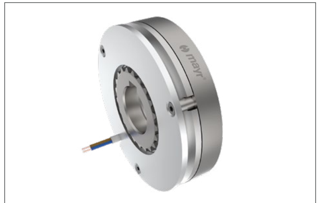
Fig. 10: ROBA ® -servostop ® Lean – Slim servo brake in a classic design – Nominal torques from 0.31 Nm to 11.5 Nm Max. speed values of up to 10500 rpm
