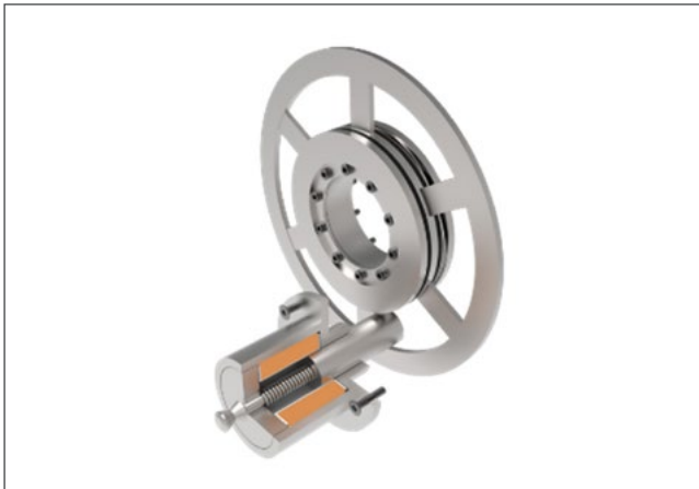
Fig. 7: Schematic layout of a pin brake. A locking pin locks the locking disk, which is firmly connected to the hollow shaft of the robot axis
