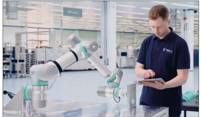
Fig. 4: Cobots can have multiple joints and degrees of freedom of movement to perform a wide range of tasks. Source: Robco
