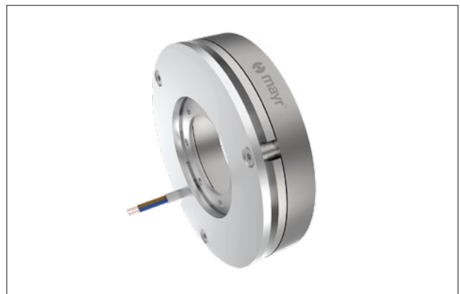
Fig. 11: ROBA ® -servostop ® Cobot – The proven series for lightweight robots, which can be integrated into even the smallest installation spaces Nominal torques from 0.23 to 9 Nm Max. speed values of up to 10500 rpm
