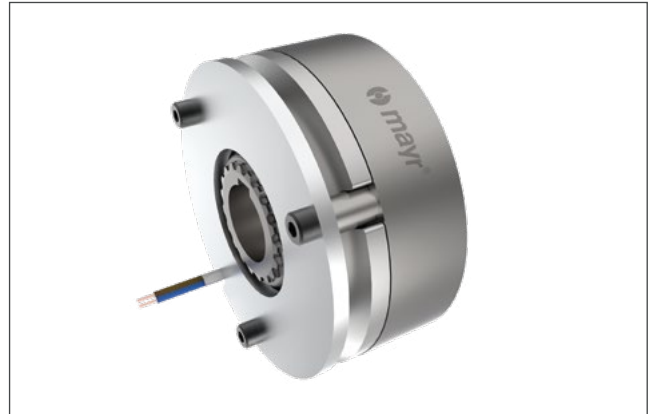
Fig. 9: ROBA ® -servostop ® Classic – Tried and tested safety brake for installation in the A or B bearing shield of servomotors Nominal torques from 1.5 to 100 Nm Max. speed values up to 9500 rpm
