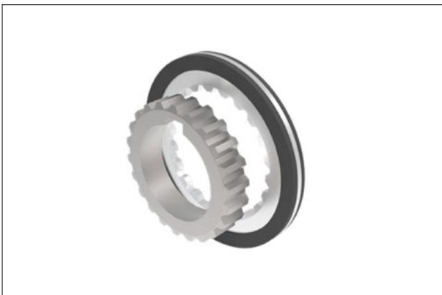
Fig. 14: The braking torque is transmitted via the internal toothing of the rotor onto the hub and via a key connection from the hub onto the shaft
